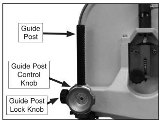
Figure 43. Guide post and lock knob.
